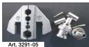
Art. 3291-05 Coaxial RG 58.59.62.6. 6.48 / 5.41 / 2.5 / 1.72 / 8.23 mm 2 0.255 / 0.213 / 0.1 / 0.68 / 0.324"
